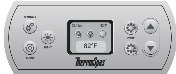
**Note:** Although the graphics on the LCD display are vivid and colorful, the screen is not a touch-screen. These menus are activated by the button located just to the side of them; such as the Light button, Jets Pump 1, Jets Pump 2, and the Up and Down buttons.
